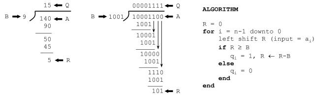
• An iterative architecture is depicted in the figure for DA with 6 bits and DB with 4 bits. The register R stores the remainder. A division operation is started when E = 1 (where DA and DB values are captured). Then, at every clock cycle, we either: i) shift in the next bit of A, or ii) shift in the next bit of A and subtract B. The signal *done* is asserted to indicate that the operation has been completed and the result appears in Q and R.
